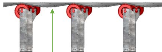
Belt sag due to lack of support
