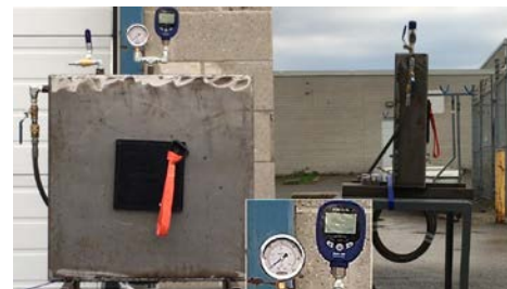
Leak Patch Pressure Test
