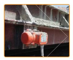
The quality of concrete can be significantly improved by vibration by reducing the volume of voids, air pockets & entrapped air in a fresh cementitious mixture.
