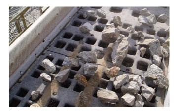
grades and profiles. They are available in standard moulds or can be custom built to shape. The properties of vulcanised rubber are dependent on the raw rubber used. Tear strength, hardness, durability, chemical and abrasion resistance are properties selected to meet the application.
