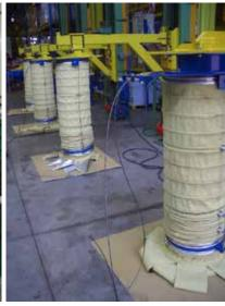
ZN Loading Bellows are used for efficient discharging of powders or granular materials into tankers.
