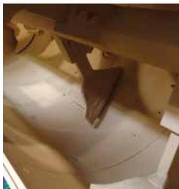
Chamber liner in special anti-wear material
