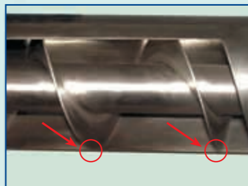
Minimum clearance between flight and tubular casing Minimaler Spalt zwischen Schneckenwendel und Rohrmantel Lumière minimum entre la spire et le tube extérieur Minima luce tra elica e tubo esterno
